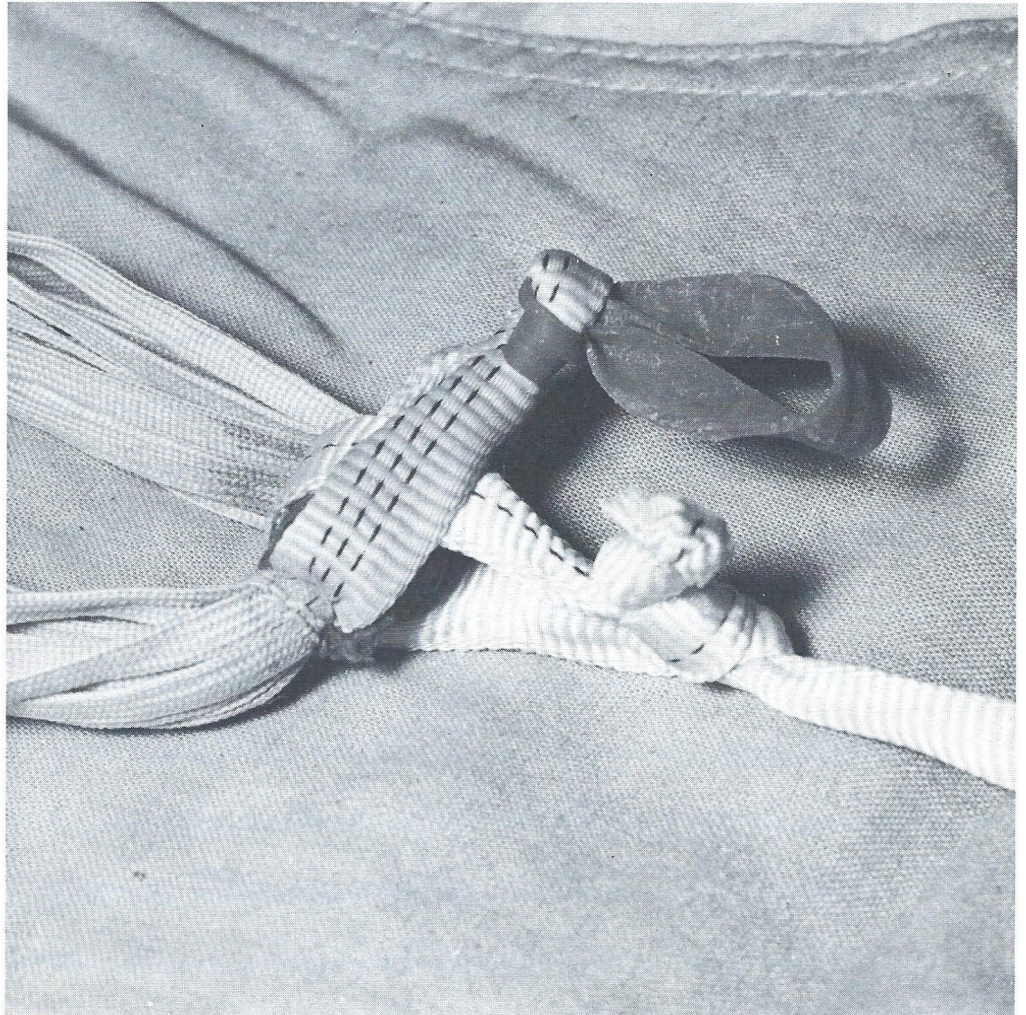
Photo 2. Clearly shows the rubber band attached to the loop at the top of the crown lines.
