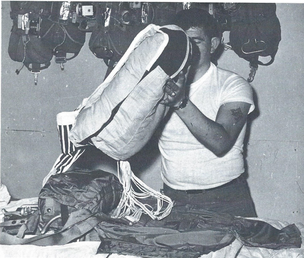
Photo 5. Towards the end of the bagging, the canopy begins to look pretty sloppy. Photo also shows how to leave the last stow in the center of the bag. Photos 6 and 7. Illustrate how the bag can be used in a Cross-Bow container. Demonstrated by Bill Van Auken.
