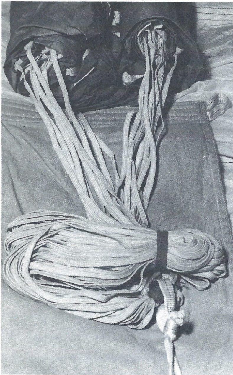
Photo 3. Crown lines "S" stowed in rubber band.
