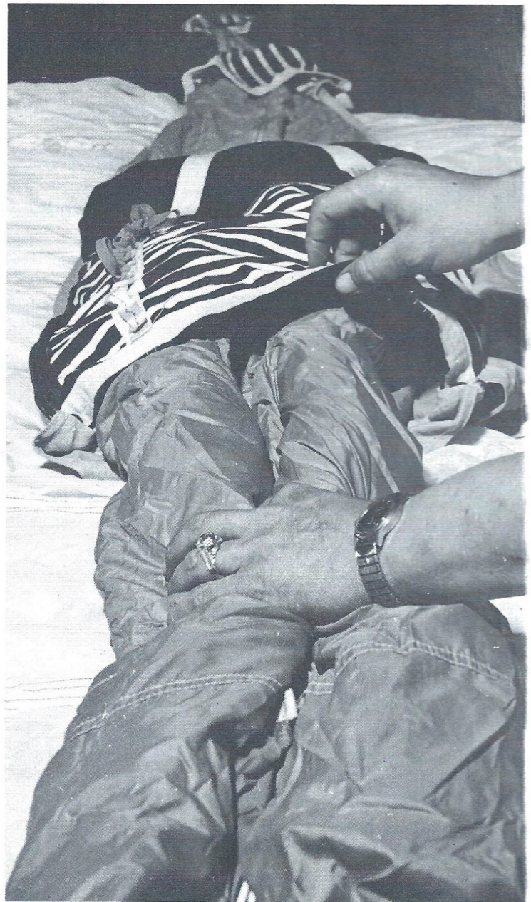
Photo 4. Canopy is "U" shaped as it is folded into the bag.
