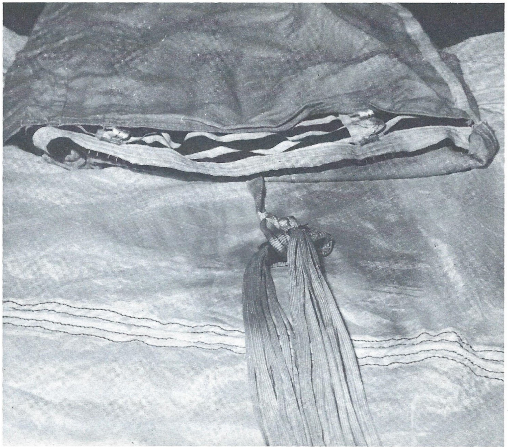
Photo 1. Illustrates how the bridled cord is attached to the crown lines.
