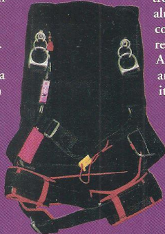
The Astra fits on the outside of the rig, near the three-ring release.
