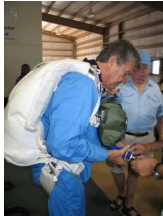
Strong Enterprises is manufacturing a one-of-a-kind parachute system, i.e., main parachute, reserve, harness and container, to be used for a new world record high-altitude freefall attempt. Strong Enterprises designed the system to be worn over a full pressure suit for the next attempt at breaking Col. Kittinger's world record freefall from 102,800 feet. Ted Strong appears above, wearing the newly designed system with a chest-mounted reserve, before
